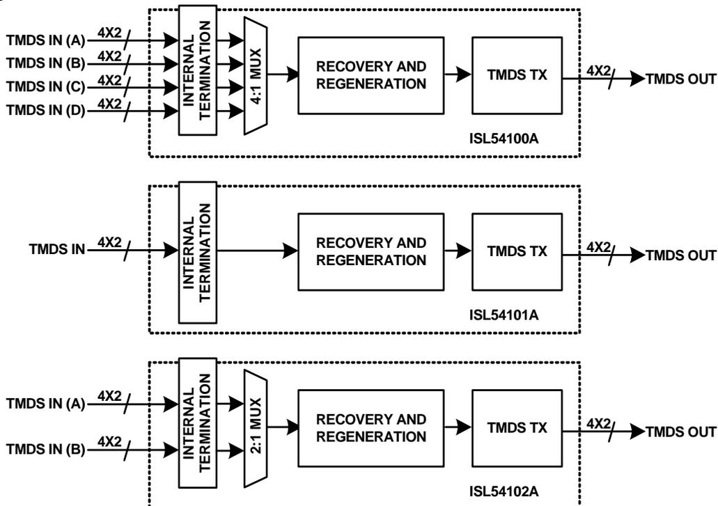
**Block Diagram of ISL54100A (ISL54101A, ISL54102A identical except for number of channels)**
