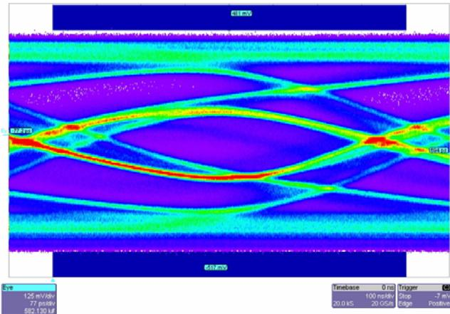
The eye is not meeting the minimum requirements of either the HDMI or DVI standards and the Dell Monitor is unable to recover the data and display an image.
