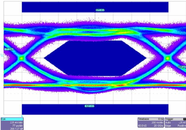
Next, a 15m DualLink DVI cable was attached and terminated into a female TPA2 adapter and the eye captured in Figure 6.
