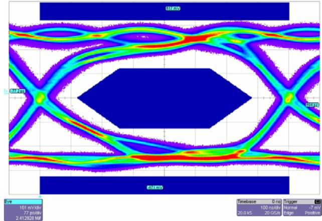
The cleaner signal generated at the output of the ISL54100A results in an improved eye at the end of another 15m cable (Figure 9). The eye is open enough that the Dell 2000FP can now display a UXGA image with no visible sparkle or other artifacts.
