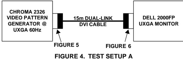
The 162.5Mpixel/s (UXGA 60Hz) DVI output of the Chroma 2326 was terminated into a TPA2 Plug adapter and measured with a LeCroy differential probe and 6MHz SDA using the LeCroy's software clock recovery. As Figure 5 shows, the amplitude of the TMDS signal is slightly low, but the eye is otherwise acceptable.
