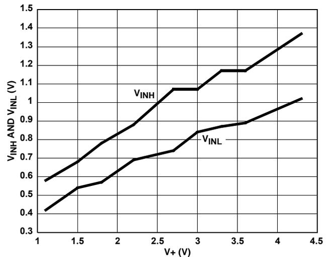
FIGURE 16. DIGITAL SWITCHING POINT vs SUPPLY VOLTAGE
