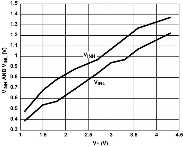
FIGURE 15. DIGITAL SWITCHING POINT vs SUPPLY VOLTAGE
