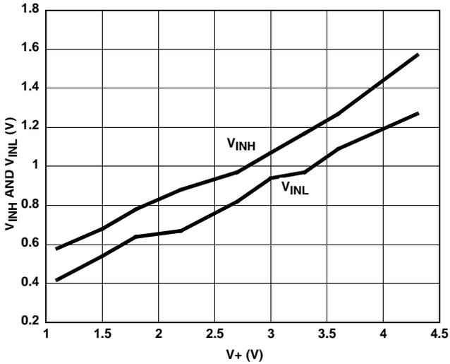
FIGURE 14. DIGITAL SWITCHING POINT vs SUPPLY VOLTAGE
