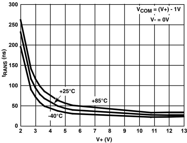
FIGURE 16. ADDRESS TRANS TIME vs SINGLE SUPPLY VOLTAGE
