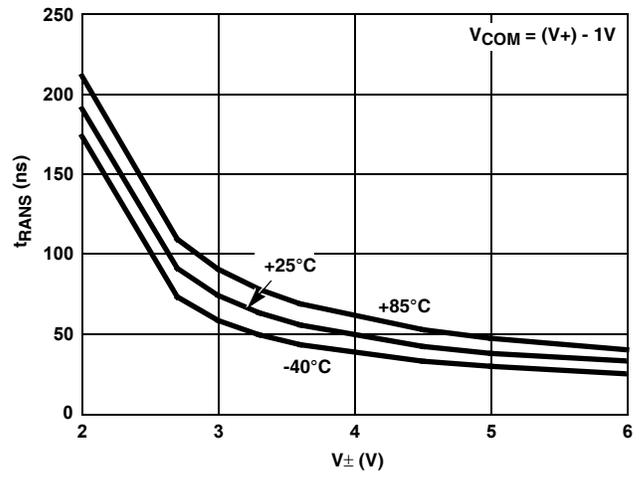
FIGURE 17. ADDRESS TRANS TIME vs DUAL SUPPLY VOLTAGE
