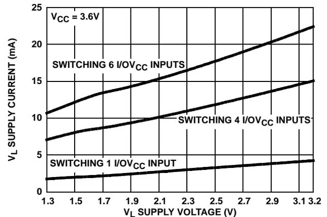
FIGURE 8. V<sub>L</sub> SUPPLY CURRENT vs V<sub>L</sub> SUPPLY VOLTAGE
