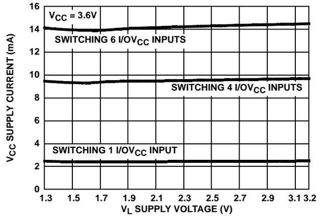
FIGURE 10.  $V_{CC}$  SUPPLY CURRENT vs  $V_L$  SUPPLY VOLTAGE
