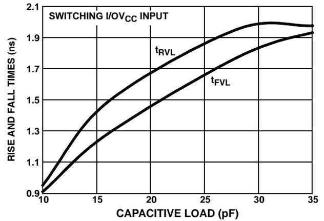
FIGURE 16. RISE/FALL TIME vs I/OV<sub>L</sub> CAPACITIVE LOAD
