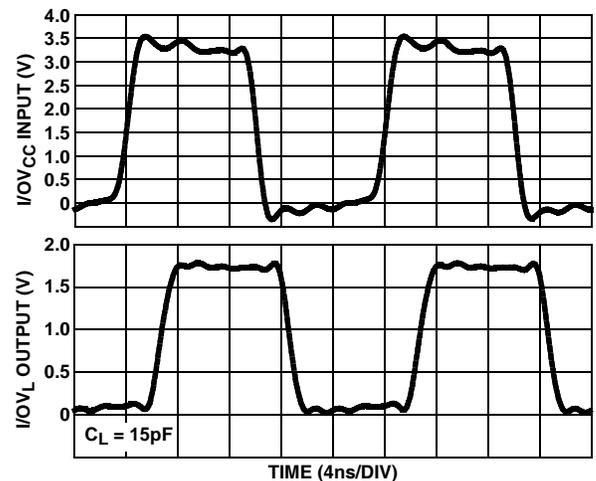
FIGURE 20. I/OV<sub>L</sub> OUTPUT WAVEFORMS (100Mbps)
