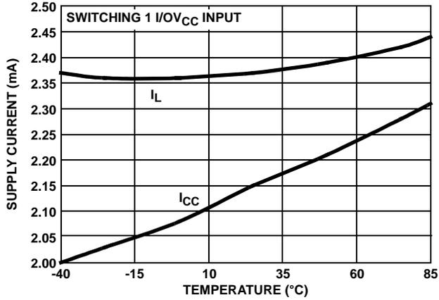
FIGURE 11. SUPPLY CURRENT vs TEMPERATURE
