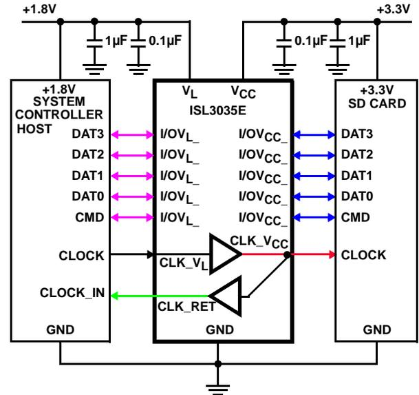
FIGURE 6. ISL3035E IN AN SD CARD APPLICATION
