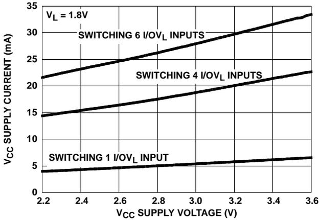
FIGURE 9.  $V_{CC}$  SUPPLY CURRENT vs  $V_{CC}$  SUPPLY VOLTAGE
