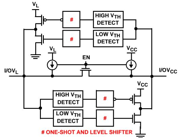
**FIGURE 5. ONE CHANNEL SIMPLIFIED SCHEMATIC**
