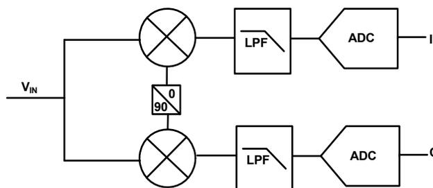
FIGURE 4. I AND Q PROCESSING OF THE SIGNAL
