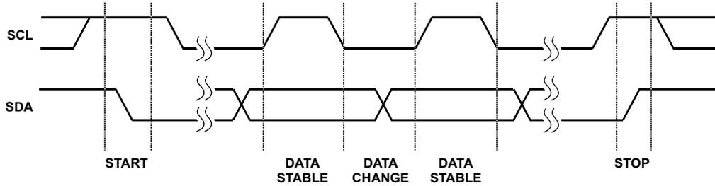
FIGURE 11. VALID DATA CHANGES, START AND STOP CONDITIONS
