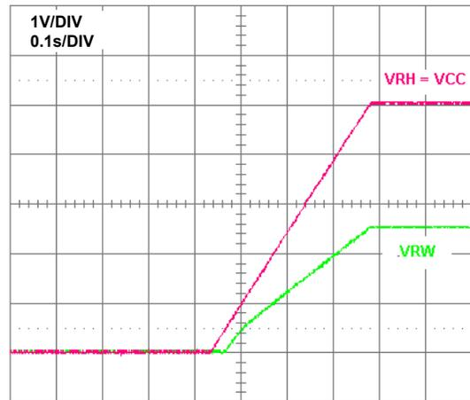
FIGURE 22. POWER-ON START-UP IN VOLTAGE DIVIDER MODE
