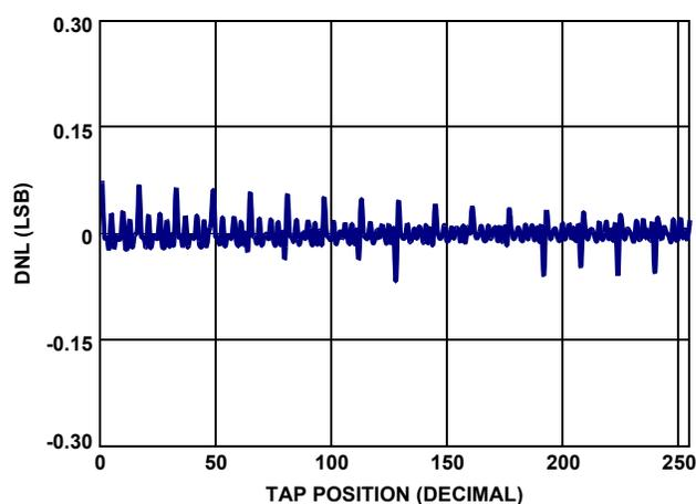
FIGURE 4. 50k DNL vs TAP POSITION,  $V_{CC} = 5V$
