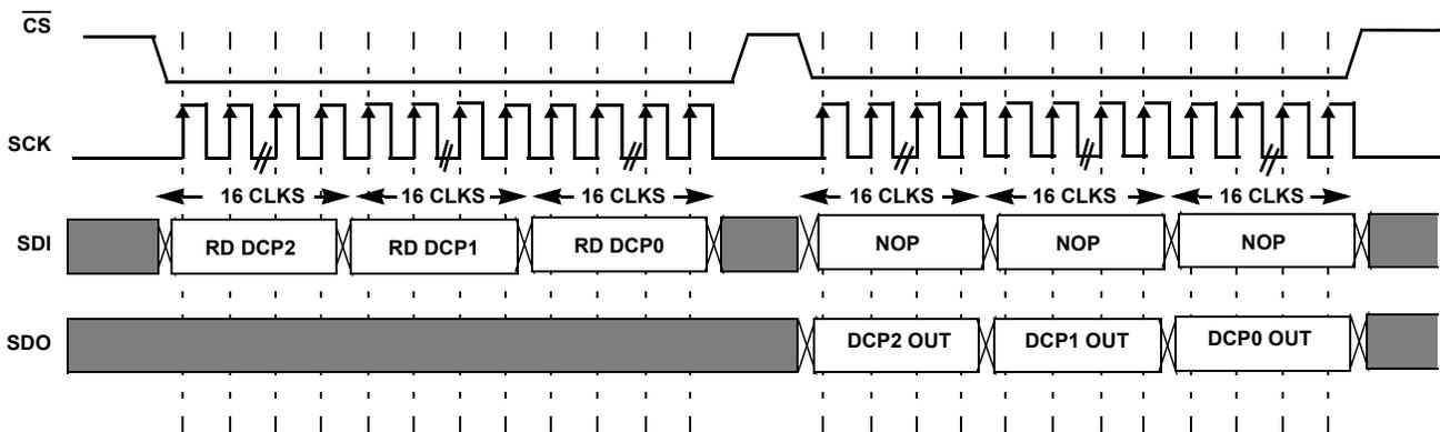
FIGURE 32. DAISY CHAIN READ SEQUENCE OF N = 3 DCP
