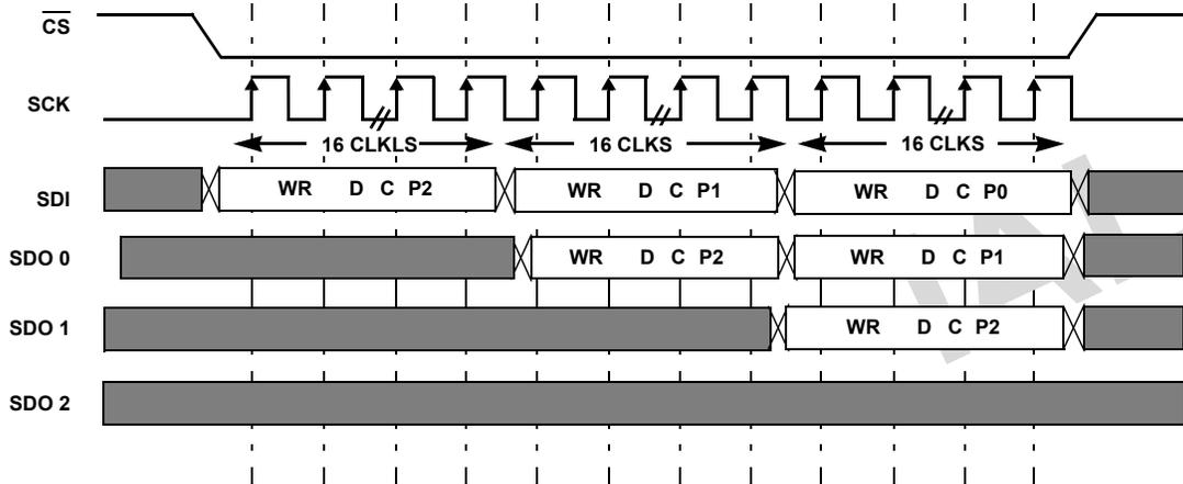
FIGURE 30. DAISY CHAIN WRITE SEQUENCE OF N = 3 DCP
