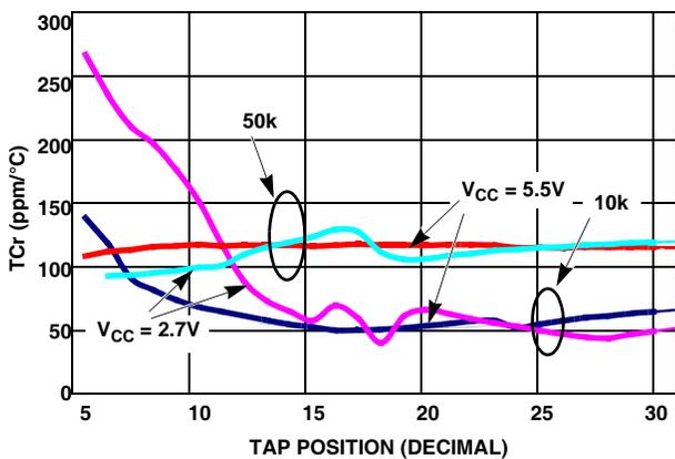
FIGURE 11. TC FOR RHEOSTAT MODE IN ppm
