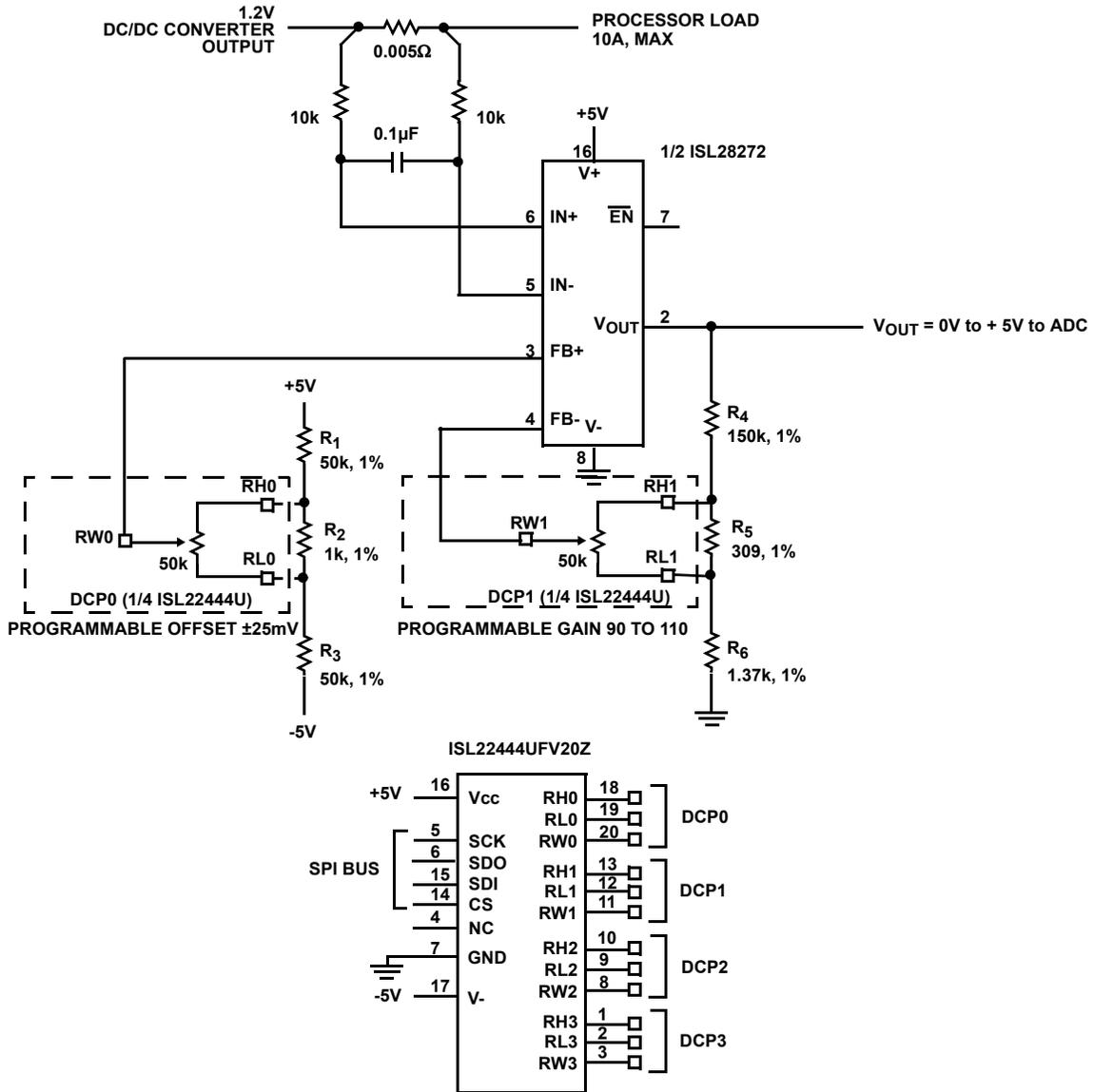
FIGURE 22. CURRENT SENSING WITH GAIN AND OFFSET CONTROL
