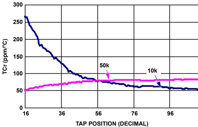
FIGURE 11. TCr FOR RHEOSTAT MODE IN ppm
