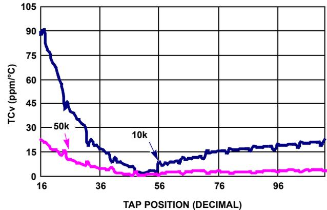
FIGURE 10. TC FOR VOLTAGE DIVIDER MODE IN ppm
