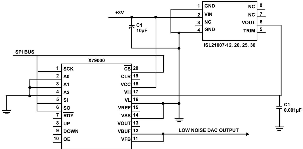
FIGURE 1. TYPICAL APPLICATION PRECISION 12-BIT SUBRANGING DAC
