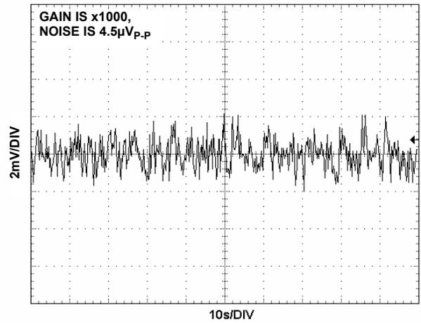
FIGURE 40. V<sub>OUT</sub> NOISE, 0.1Hz TO 10Hz
