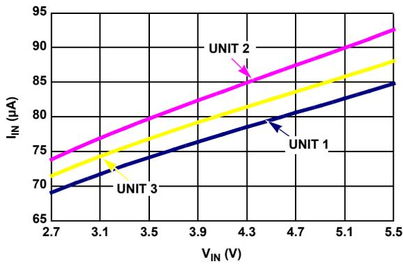
FIGURE 15.  $I_{IN}$  vs  $V_{IN}$  (3 UNITS)
