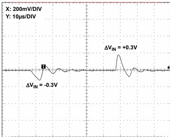
FIGURE 23. LINE TRANSIENT RESPONSE, 0.001 $\mu$ F LOAD CAPACITANCE
