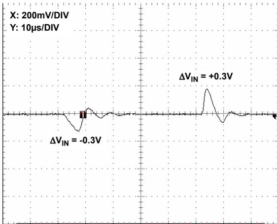
FIGURE 10. LINE TRANSIENT RESPONSE, 0.001μF LOAD CAPACITANCE
