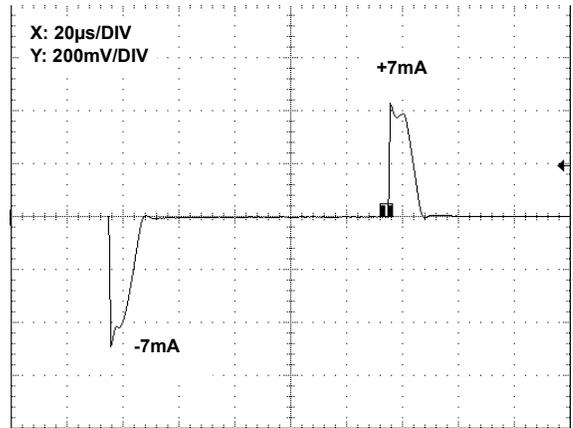
FIGURE 28. LOAD TRANSIENT RESPONSE, NO CAPACITIVE LOAD
