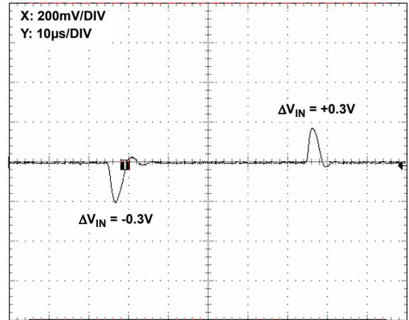
FIGURE 22. LINE TRANSIENT RESPONSE, NO CAPACITIVE LOAD
