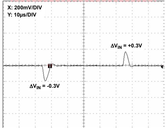
FIGURE 9. LINE TRANSIENT RESPONSE, NO CAPACITIVE LOAD
