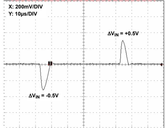
FIGURE 49. LINE TRANSIENT RESPONSE, NO CAPACITIVE LOAD
