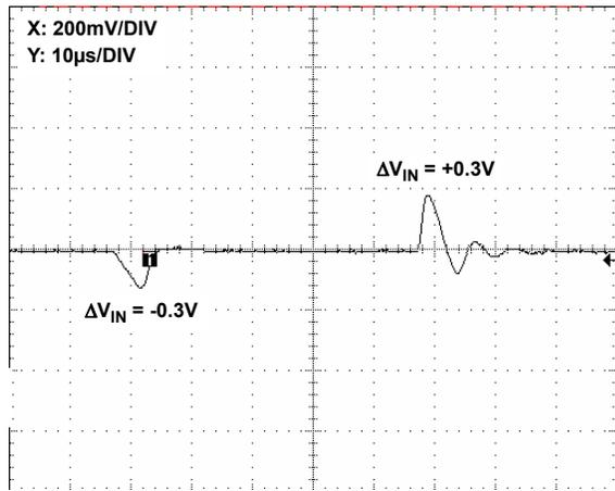
FIGURE 37. LINE TRANSIENT RESPONSE, 0.001µF LOAD CAPACITANCE
