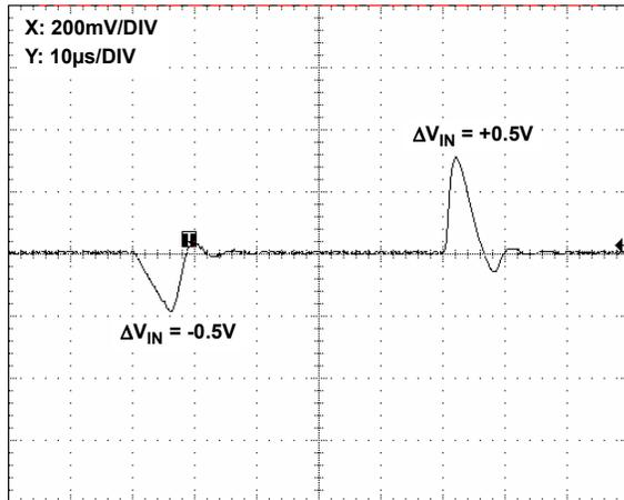
FIGURE 50. LINE TRANSIENT RESPONSE, 0.001μF LOAD CAPACITANCE
