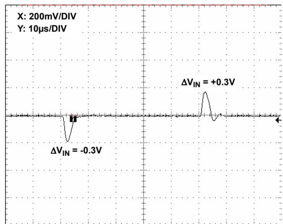
FIGURE 36. LINE TRANSIENT RESPONSE, NO CAPACITIVE LOAD
