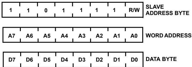
FIGURE 17. SLAVE ADDRESS, WORD ADDRESS, AND DATA BYTES
