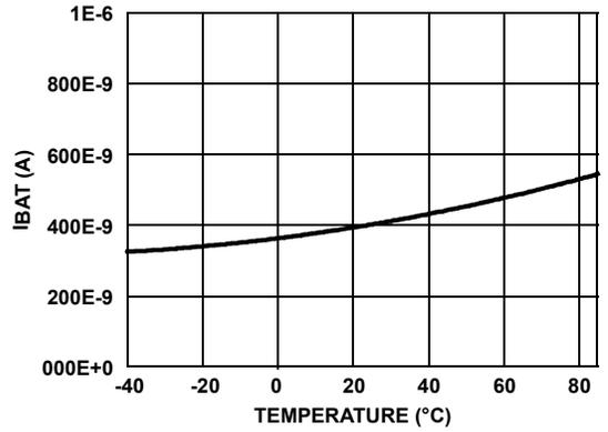
FIGURE 2. I<sub>BAT</sub> vs TEMPERATURE AT V<sub>BAT</sub> = 3V
