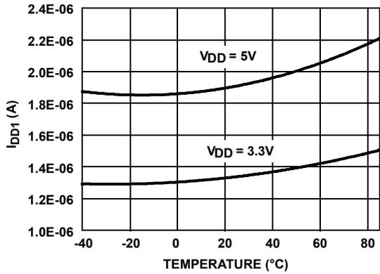
FIGURE 3. I<sub>DD1</sub> vs TEMPERATURE
