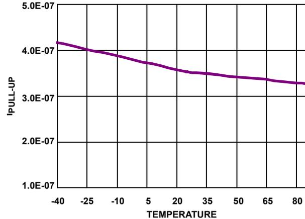
FIGURE 8.  $I_{PULLUP}$  vs TEMPERATURE AT  $V_{BAT} = 1.8V$ EQUIVALENT AC OUTPUT LOAD CIRCUIT FOR  $V_{DD} = 5V$
