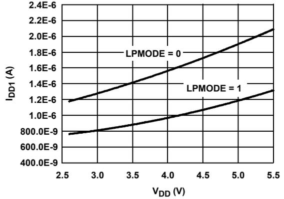
FIGURE 4. I<sub>DD1</sub> vs V<sub>DD</sub> WITH LPMODE ON AND OFF
