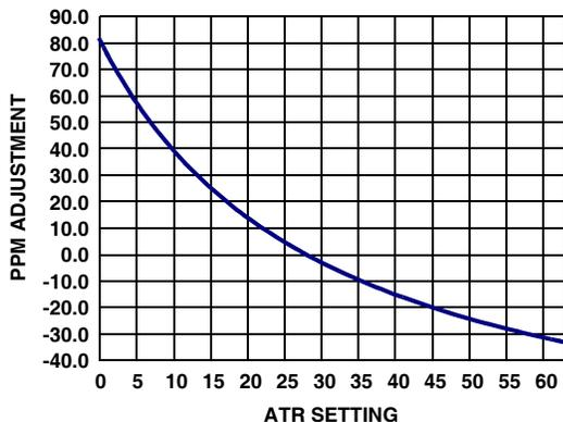
FIGURE 21. ATR SETTING vs. OSCILLATOR FREQUENCY ADJUSTMENT
