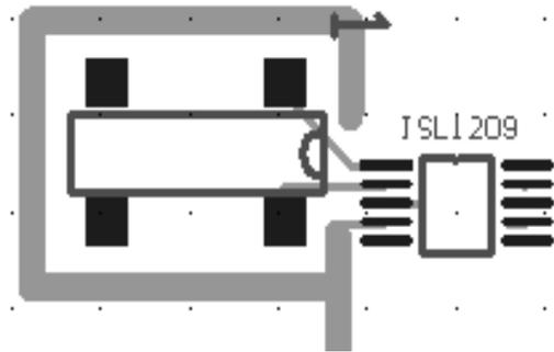
FIGURE 20. SUGGESTED LAYOUT FOR ISL1209 AND CRYSTAL
