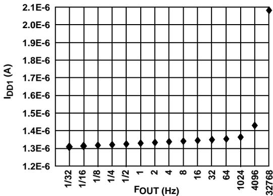
FIGURE 5. I<sub>DD1</sub> vs F<sub>OUT</sub> AT V<sub>DD</sub> = 3.3V
