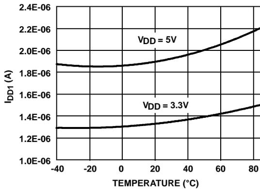
FIGURE 3. I<sub>DD1</sub> vs TEMPERATURE
