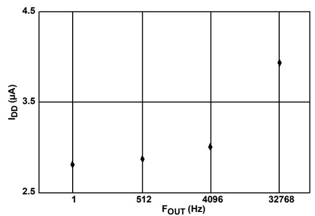
FIGURE 6. I<sub>DD1</sub> vs f<sub>OUT</sub> AT V<sub>DD</sub> = 5V
