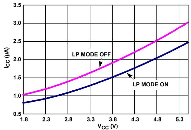
FIGURE 4. I<sub>DD1</sub> vs V<sub>CC</sub> WITH LPMODE ON AND OFF
