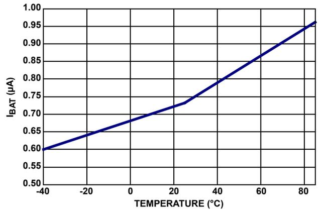
FIGURE 2. I<sub>BAT</sub> vs TEMPERATURE AT V<sub>BAT</sub> = 3V
