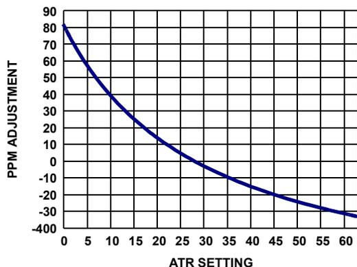
FIGURE 18. ATR SETTING vs OSCILLATOR FREQUENCY ADJUSTMENT
