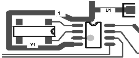
FIGURE 19. SUGGESTED LAYOUT FOR ISL12082 AND CRYSTAL
