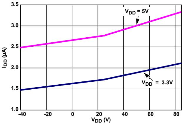
FIGURE 3. I<sub>DD1</sub> vs TEMPERATURE
