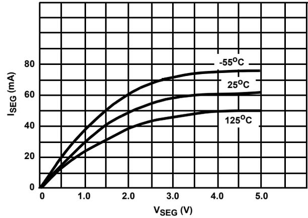
FIGURE 6. COMMON ANODE SEGMENT DRIVER  $I_{SEG}$  vs  $V_{SEG}$
