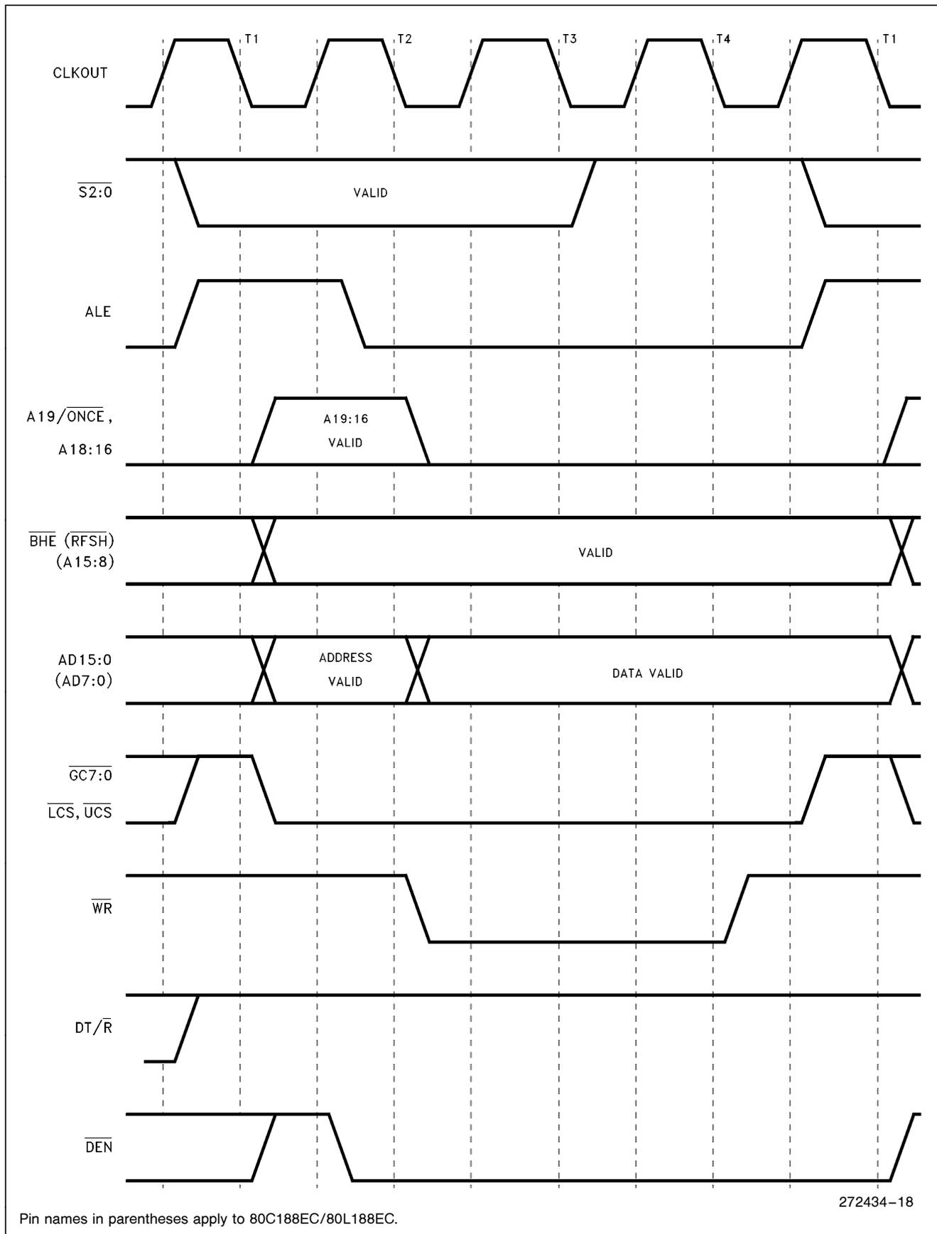
Figure 19. Memory Write and I/O Write Cycle Waveforms
