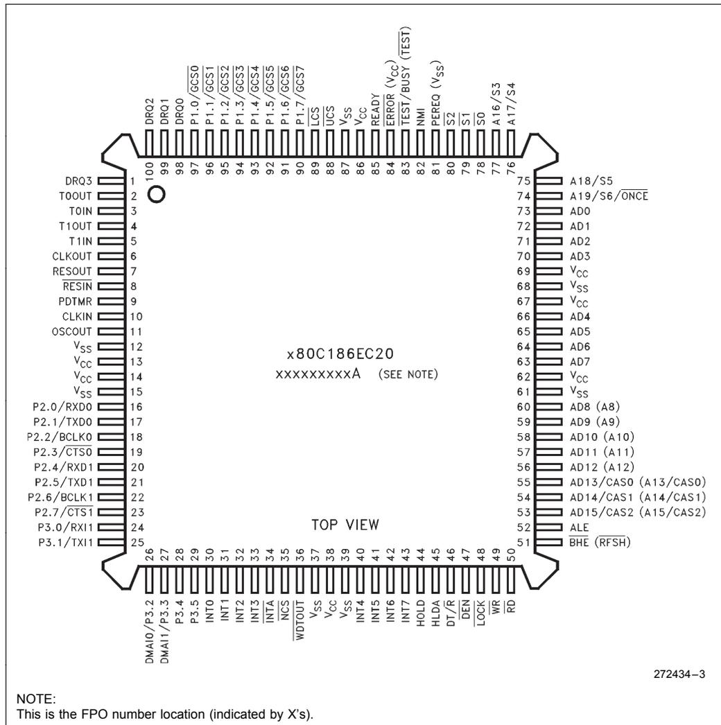
Figure 4. 100-Pin Plastic Quad Flat Pack Package (PQFP)
