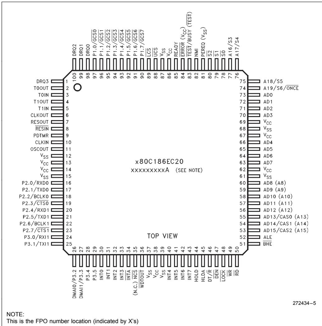
Figure 6: 100-Pin Shrink Quad Flat Pack Package (SQFP)
