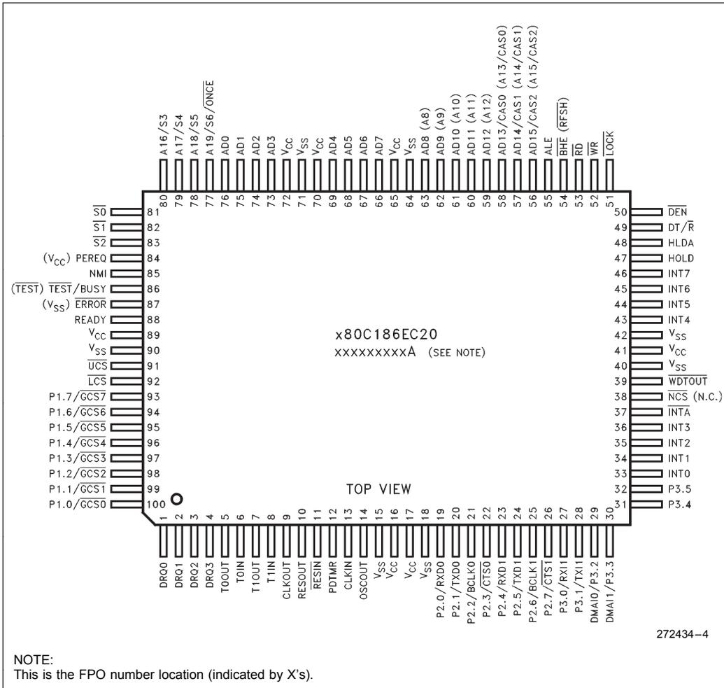
Figure 5: Quad Flat Pack (EIAJ) Pinout Diagram
