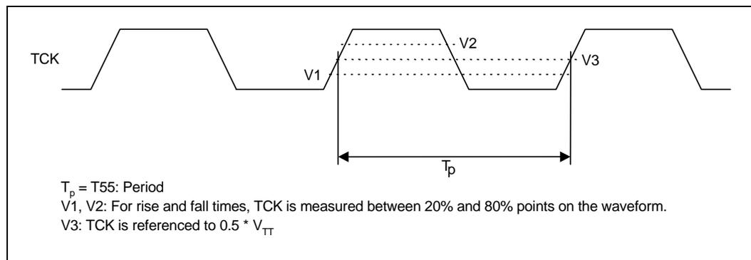
Figure 2-15. Differential Clock Waveform
