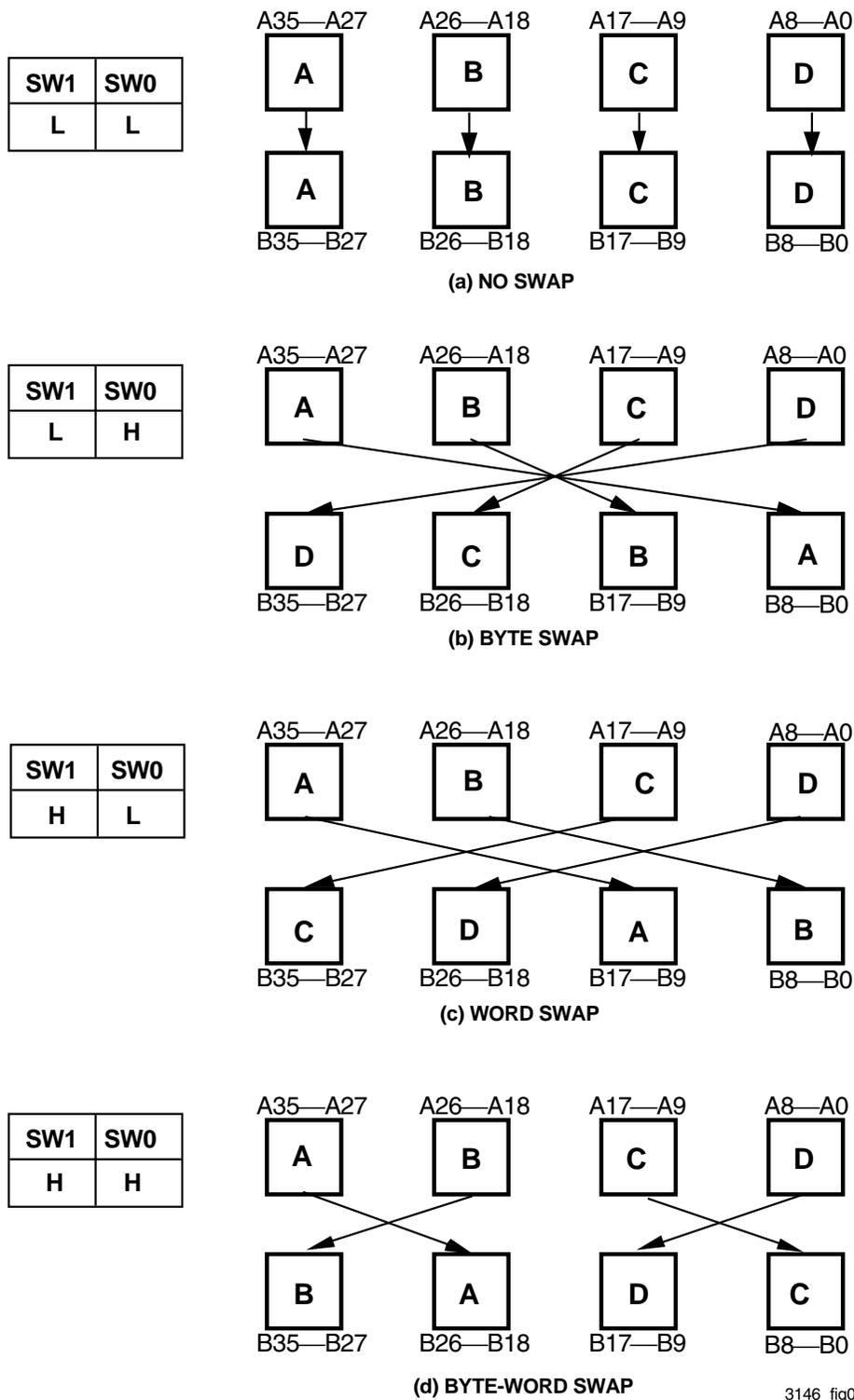
Figure 4. Byte Swapping (Long Word Size Example)
