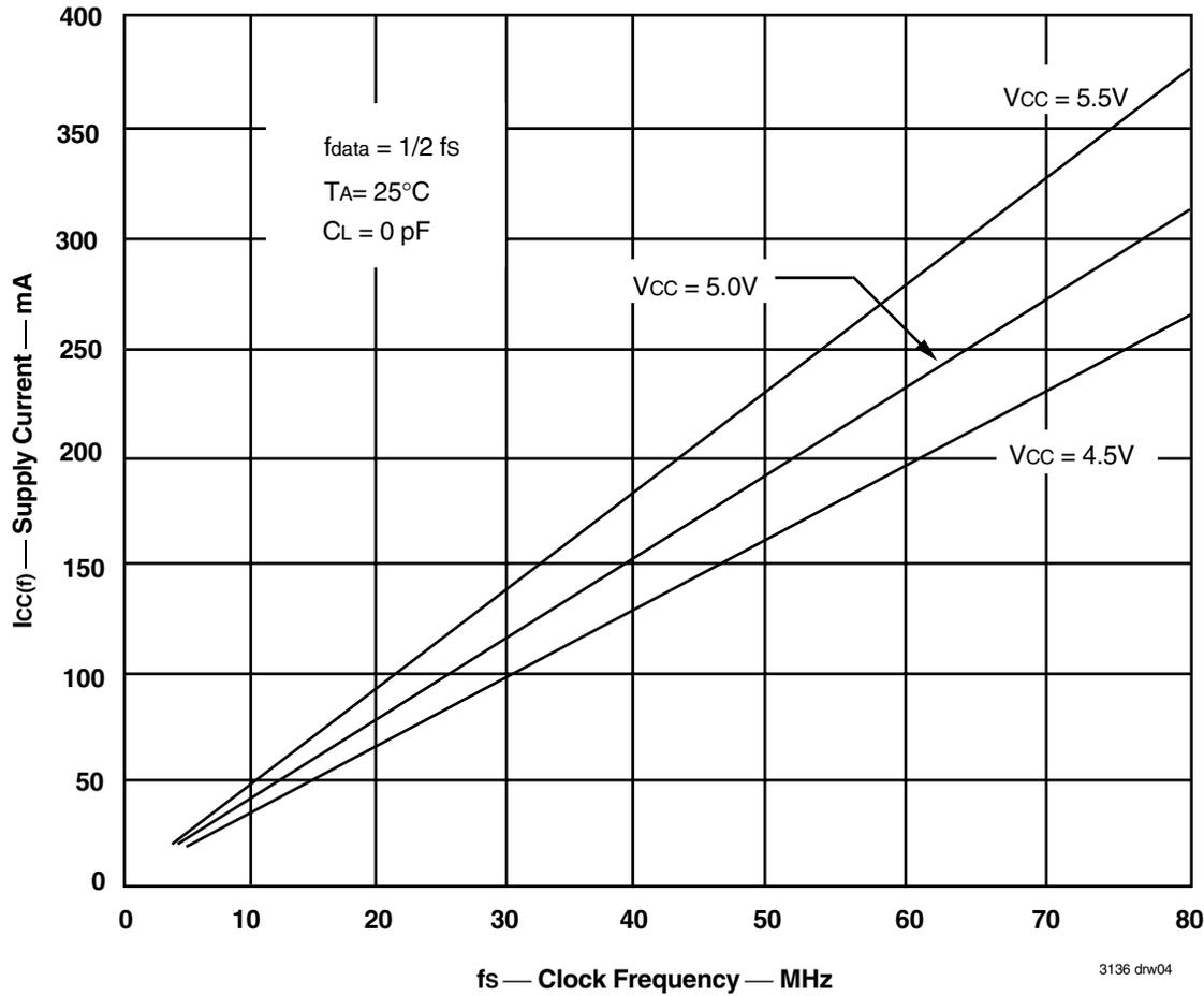
Figure 1. Typical Characteristics: Supply Current vs Clock Frequency
