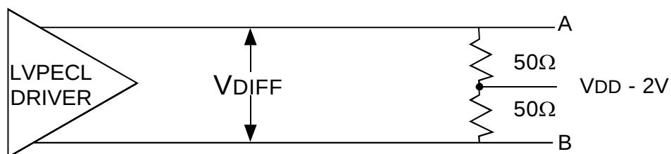
Test Circuit for LVPECL Output Characteristics
