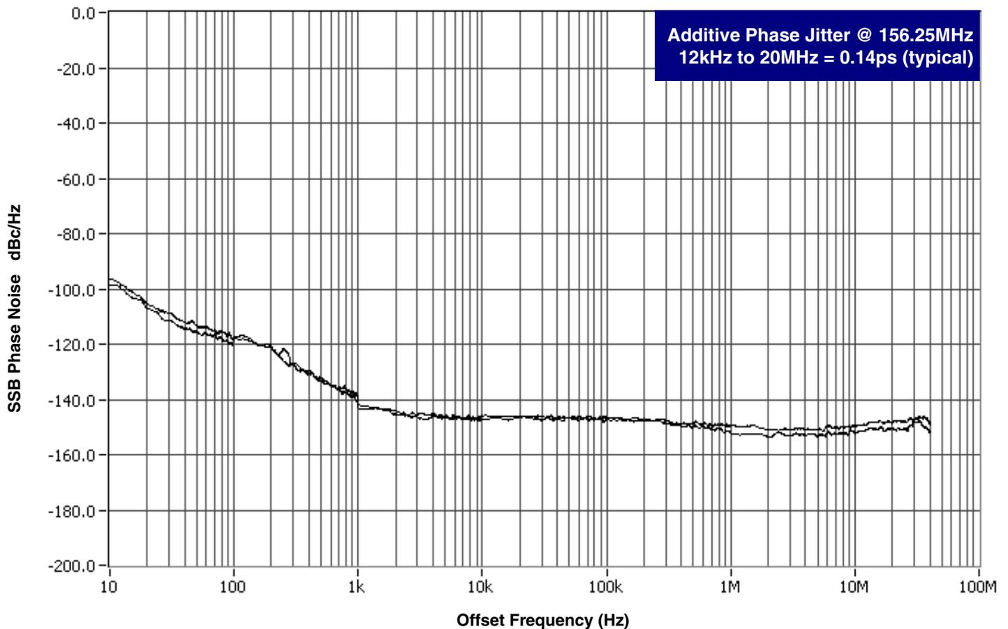
As with most timing specifications, phase noise measurements has issues relating to the limitations of the equipment. Often the noise floor of the equipment is higher than the noise floor of the
