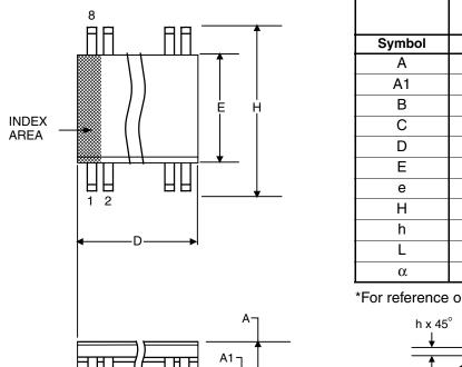
Millimeters Inches\* Min Max Min Max .0532 .0688 1.35 1.75 0.10 0.25 .0040 .0098 0.33 0.51 .013 .020 0.19 0.25 .0075 .0098 4.80 5.00 .1890 .1968 3.80 4.00 .1497 .1574 1.27 BASIC 0.050 BASIC 6.20 .2284 .2440 5.80 0.25 0.50 .010 .020 0.40 1.27 .016 .050 0° 0° 8° 8°
