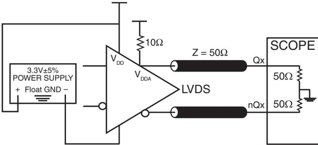
LVDS 3.3V OUTPUT LOAD TEST CIRCUIT
