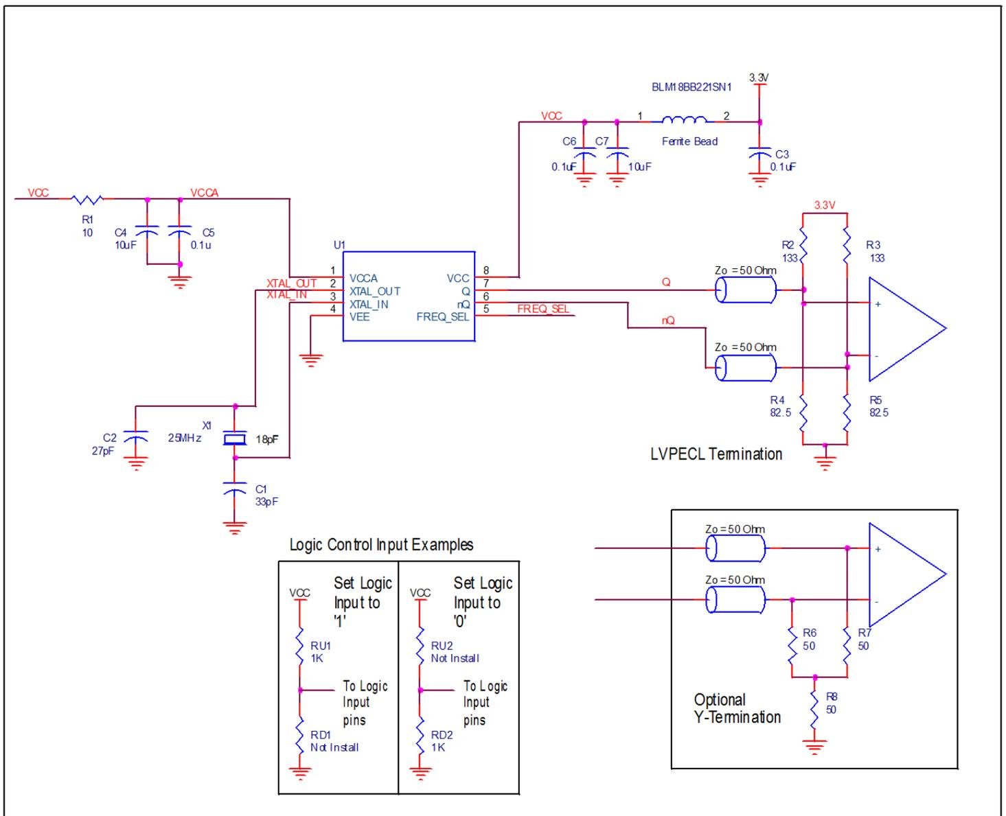
Figure 6. 843071 Application Schematic
