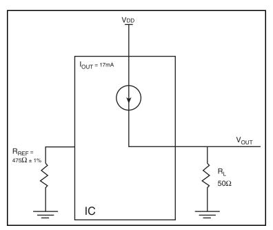
Figure 4. HCSL Driver Circuit and Termination
