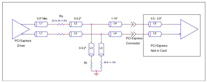
Figure 3A. Recommended Source Termination (where the driver and receiver will be on separate PCBs)
