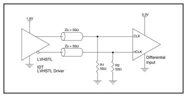
Figure 2A. CLK/nCLK Input Driven by an IDT Open Emitter HiPerClockS LVHSTL Driver
