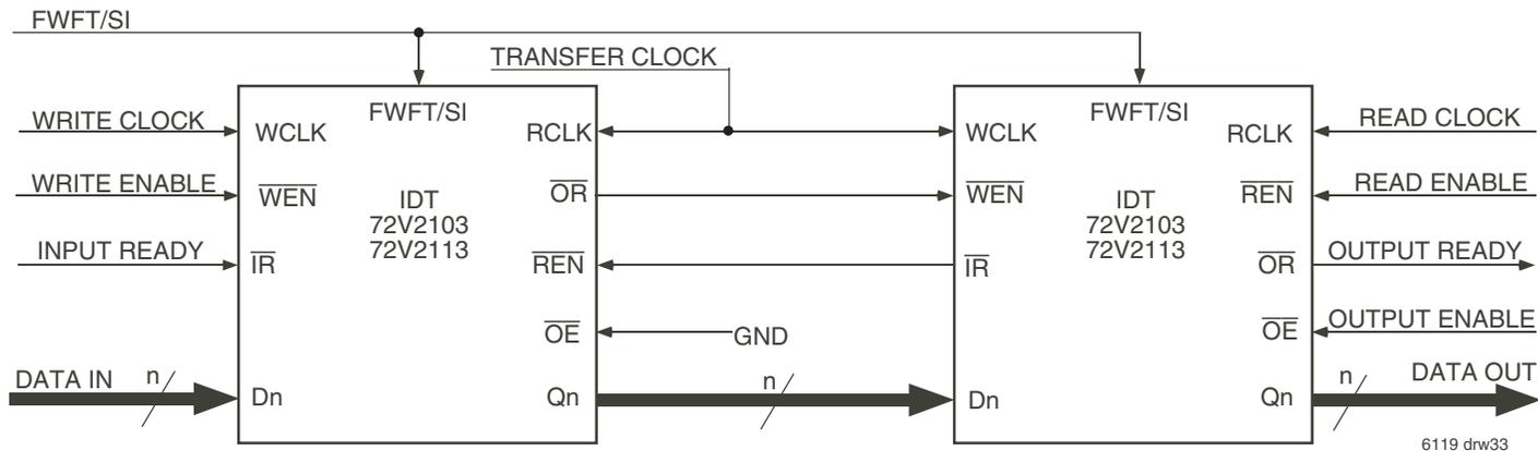
**Figure 30. Block Diagram of Depth Expansion**
