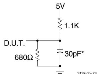
**Figure 1. Output Load**
