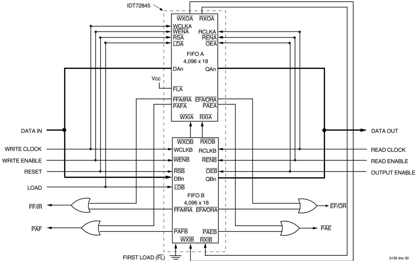
*Figure 30. Block Diagram of 8,192 x 18 Synchronous
