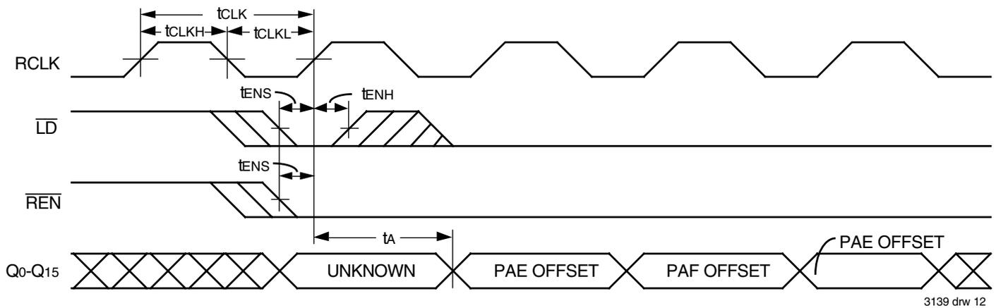
Figure 12. Read Programmable Registers (IDT Standard Mode)
