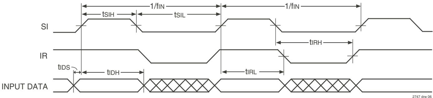
Figure 2. Input Timing
