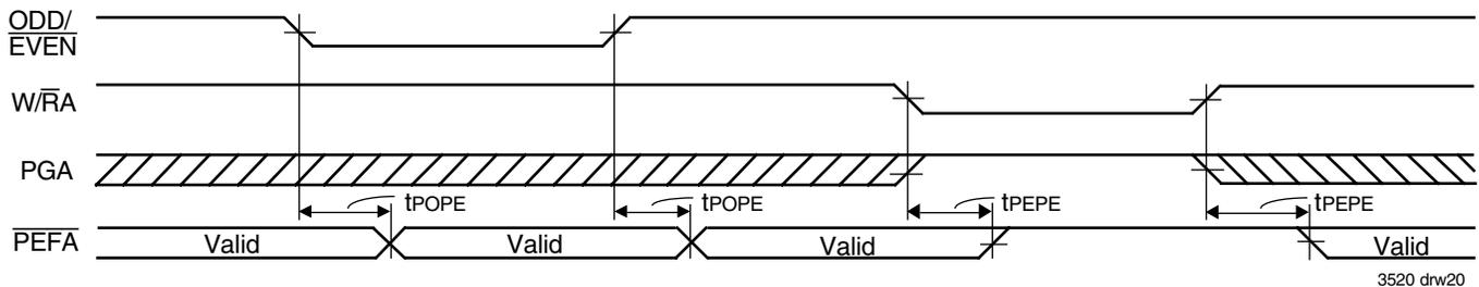
Figure 20. ODD/EVEN, WRA and PGA to PEFA Timing
