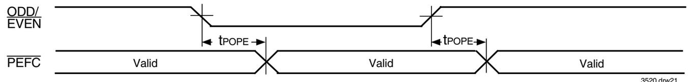
Figure 21. ODD/EVEN to PEFC Timing
