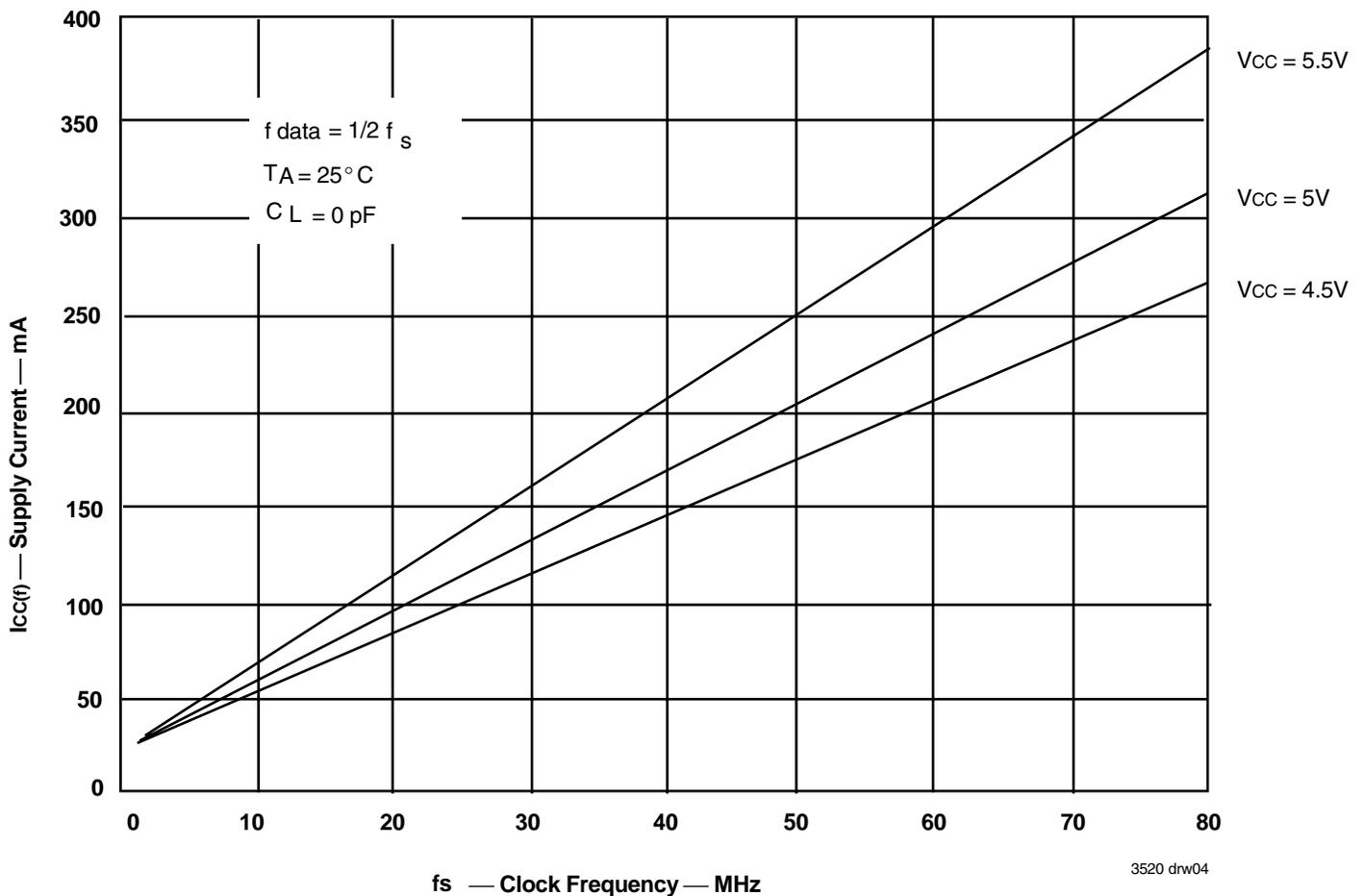
Figure 1. Typical Characteristics: Supply Current vs Clock Frequency
