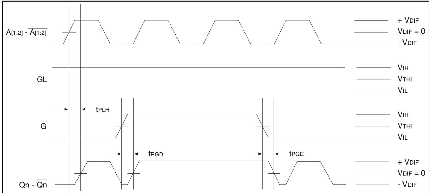
NOTE 1: As shown, it is possible to generate runt pulses on gate disable and enable of the outputs. It is the user's responsibility to time the  $\overline{G}$  signal to avoid this problem.
