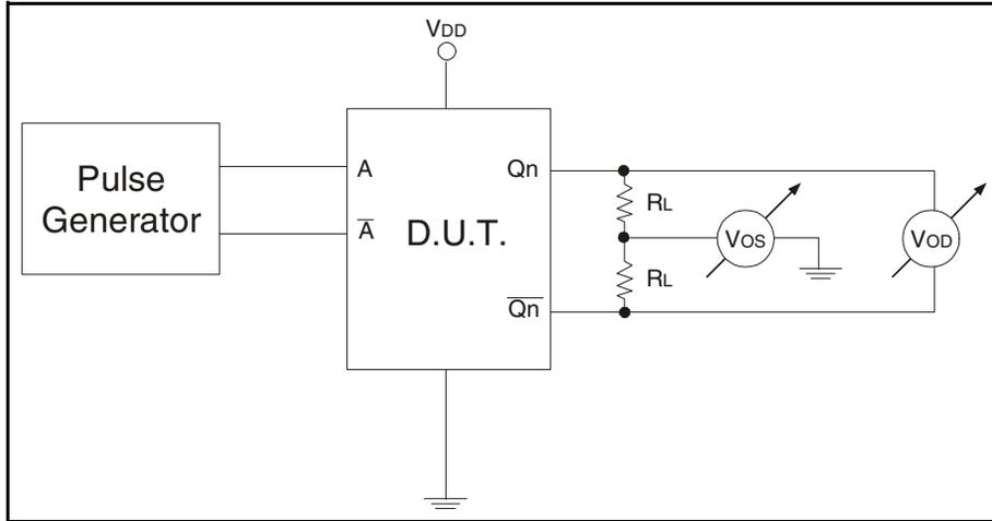
**Test Circuit for Propagation, Skew, and Gate Enable/Disable Timing**
