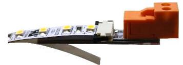
**5** Make sure LED strip is centered and fully inserted before sliding black latch firmly closed and pressing on adhesive.
