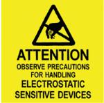
This InnoSenT sensor is sensitive to damage from ESD. Normal precautions as usually applied to CMOS devices are sufficient when handling the device. Touching the signal output pins has to be avoided at any time before soldering or plugging the device into a motherboard.
