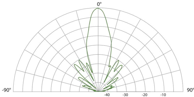
Elevation (measured @61GHz)
