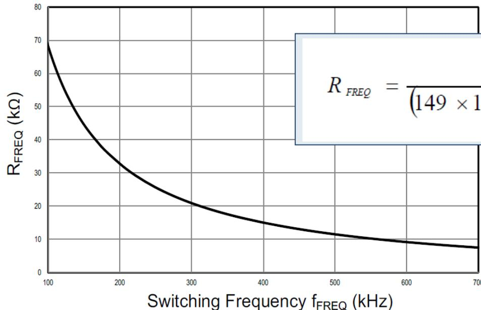
$$R_{FREQ} = \frac{1}{(149 \times 10^{-12} [\frac{s}{\Omega}]) \times (f_{FREQ} [\frac{1}{s}])} - (2.0 \times 10^3 [\Omega]) [\Omega]$$
