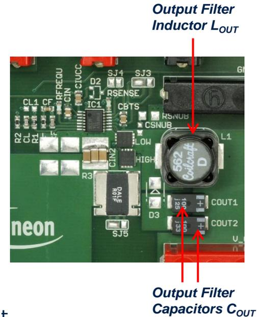
$$(1) \quad \Delta I_{ripple} = \frac{(V_{IN} - V_{OUT})V_{OUT}}{L_{OUT} f_{SW} V_{IN}}$$
