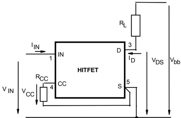
The ground lead impedance of  $R_{CC}$  should be as low as possible
