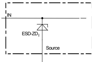
ESD zener diodes are not designed for DC current  $> 2 \text{ mA}$  @  $V_{IN} > 10\text{V}$ .
