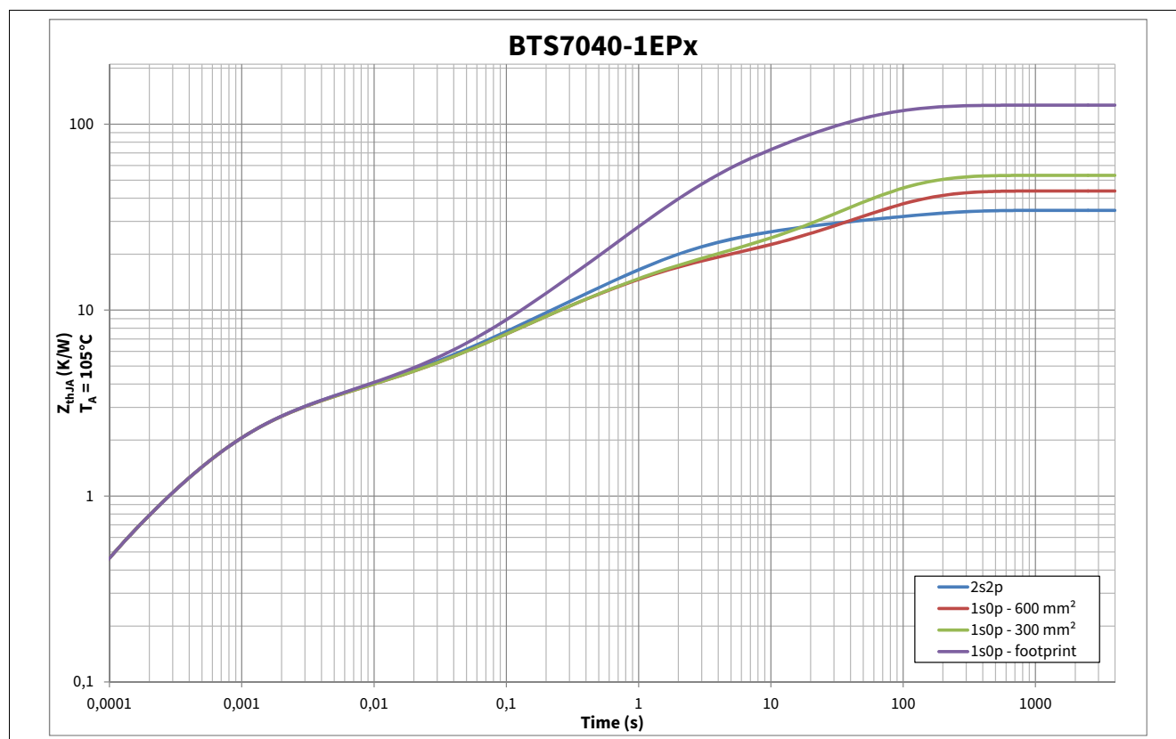
Figure 9 Typical Thermal Impedance. PCB setup according Chapter 4.4.1
