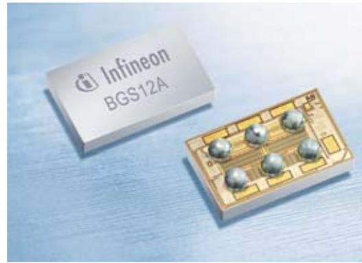
THE BGS12A is Infineon's first product in its new Radio Frequency (RF) switch family. The BGS12A is a general purpose Single-Pole, Double-Throw (SPDT) RF switch, designed for power levels of up to 20dBm, with a P-1dB above 30dBm.
