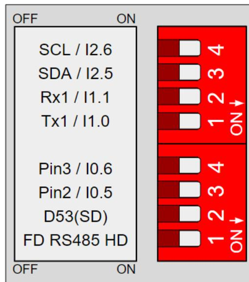
**4. SCL/I2.6: ALWAYS AT OFF POSITION.** On the MDUINO PLC ARDUINO ETHERNET & WIFI & BLE 38AR I/Os ANALOG/DIGITAL PLUS Controller this switch is **not connected**.
