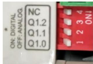
For the Relay Shield if a switch is set to ON, it can only act as Digital Output. If it is set to OFF it can only act as an Analog Output.
