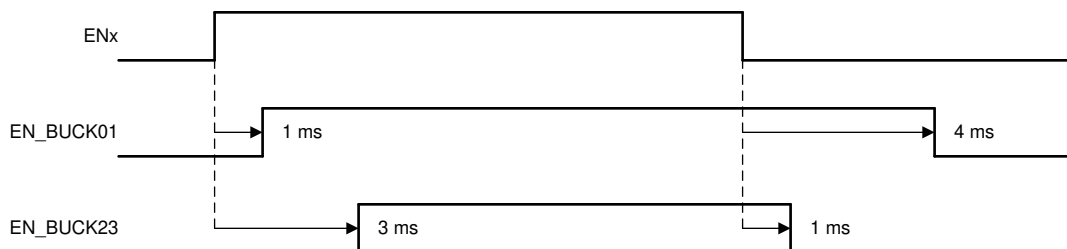
Figure 10. Typical Start-Up and Shutdown Sequencing
