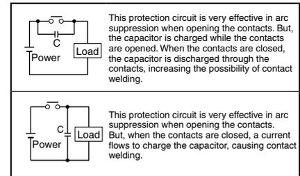
Generally, switching a DC inductive load is more difficult than switching a DC resistive load. Using an appropriate arc suppressor will improve the switching characteristics of a DC inductive load.
