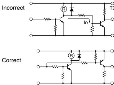
When driving an element at the same time as the relay operation, special consideration is needed for the circuit design. As shown in the incorrect circuit below, leakage current ( $I_o$ )
