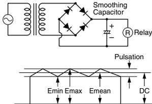
$$\text{Ripple Factor (\%)} = \frac{E_{\max} - E_{\min}}{E_{\text{mean}}} \times 100\%$$
