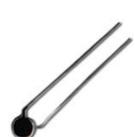
143 Series, 5,08 mm [0.2 in] disc thermistor with leads, 3,000 Ohm resistance, ±10.0% tolerance, 25/85 BETA = 3974
