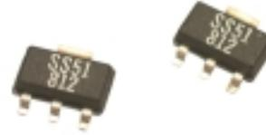
SS5 Series Hall effect position sensors are operated by the magnetic field from a permanent magnet or electromagnet. The small SOT89 style package surface mounts on PC boards and flexible circuits. The SS5 uses a industry standard "gull-wing" design which makes it less susceptible to "solder bridging" and allows increased circuit board density. The SS5 series package can accommodate larger IC's than SS1 and allows for four-pin designs
