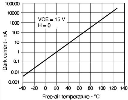
Fig. 4 Collector Current vs Ambient Temperature
