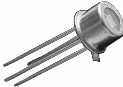
The GFD3500-002 is a high-speed optical receiver designed for data transmission in industrial LAN applications. The monolithic CMOS (Complementary Metal-Oxide Semiconductor) chip consists of a large area photodiode, pre-amplifier with controlled gain, a post-amplifier, a comparator and TTL output stage. The integrated voltage regulator provides easy use in many applications.
