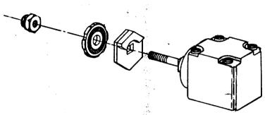
ADJUSTABLE TO OPERATE CLOCKWISE, COUNTER-CLOCKWISE, OR IN BOTH DIRECTIONS.
