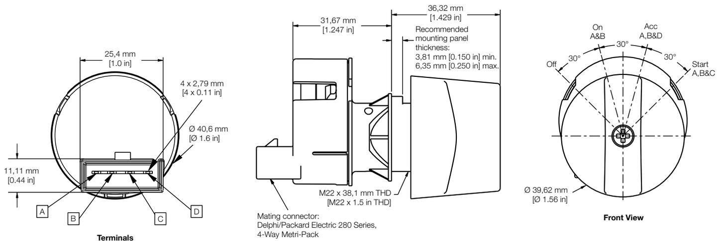
Figure 2. Model 90233 Rotary Switch Dimensions
