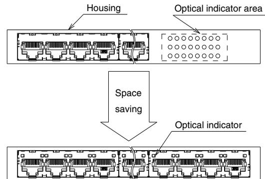
One additional TM21 multi-port jack can be mounted in the space previously occupied by LEDs.
