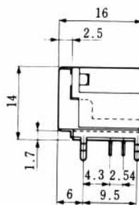
Board mounting dimensional drawing (connector side)
