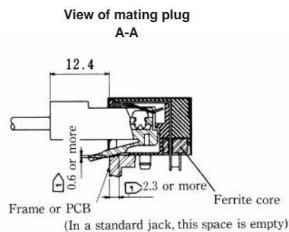
**Reference mounting dimensions (PCB component side)**
