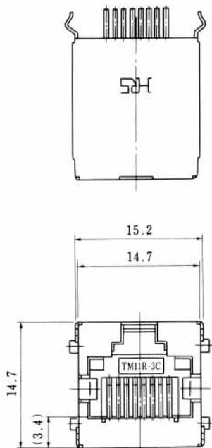
Board mounting dimensional drawing (connector side)
