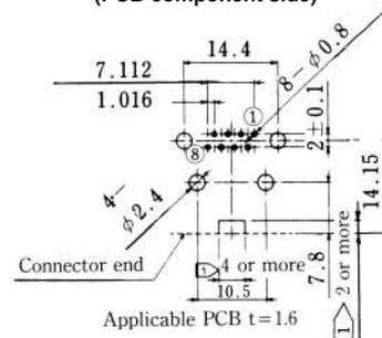
Note : When preparing frames or PCBs, provide the above for the connector.
