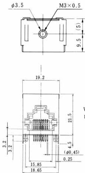
Board mounting dimensional drawing (connector side)
