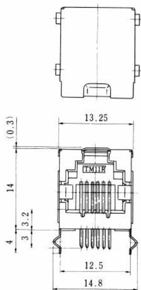
Board mounting dimensional drawing (connector side)
