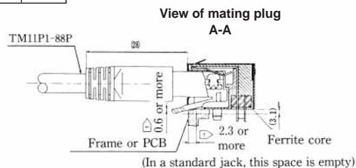
**Reference mounting dimensions (PCB component side)**
