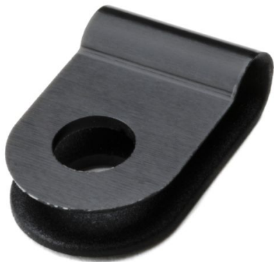
P-Clamp, 0.39" Wide, 0.13" Max Bundle Dia, 0.17" Mounting Hole Dia, PA66HS, Black, 1000/pkg
